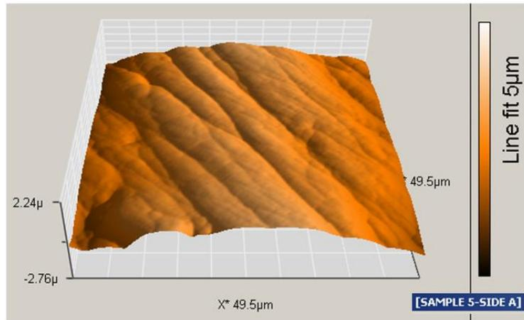
*Fig. 44 Test sample 12: Lithium disilicate press ceramics – glazed, treated with green diamond bur, polished with rubbers and diamond paste*
