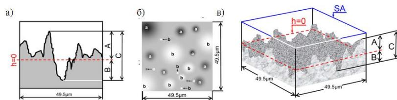
Fig. 14 Topographic image of a surface (a), image of measuring points (b), three-dimensional image of a surface (c), where SA – working area;  $h$  – level of the reference plane; A – protrusions; B – indentations; C – maximum roughness  $C = A + B$ ; a – protrusions; b – indentations.
