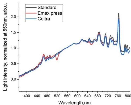
*Fig. 22 Normalized reflection spectra ( $\lambda_{norm}=560$  nm, corresponding to the maximum sensitivity of the human eye) of the studied ceramics and standard material for testing the reflective properties of solid materials of SHIMADZU, Japan.*
