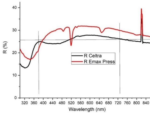
*Fig. 19 Measured reflection coefficients of ceramic materials*
