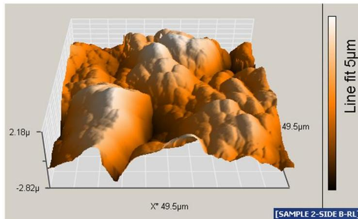
Fig. 33 Test sample 1: lithium silicate press ceramics (Celtra Press) – laboratory polished
