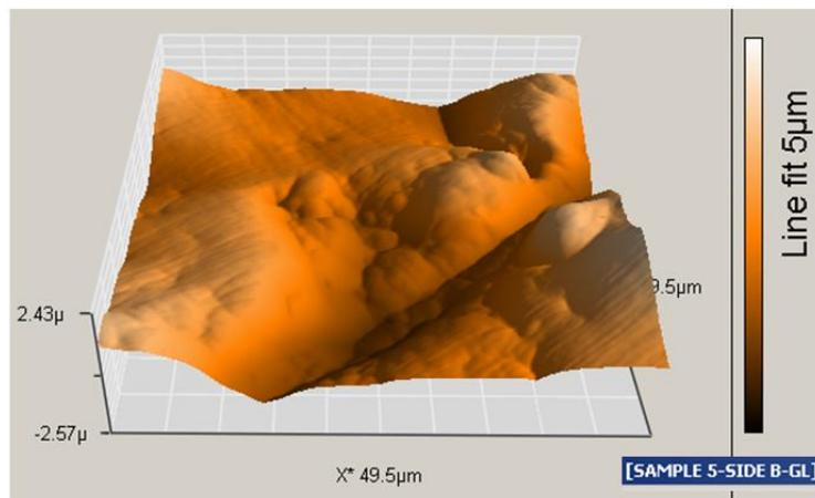
*Fig. 40 Test sample 8: Lithium disilicate pressceramics – glazed, treated with green diamond bur, polished with rubbers.*
