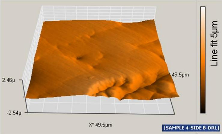
*Fig. 37 Test sample 5: Lithium silicate press ceramics – glazed, treated with red diamond bur, polished with rubbers.*
