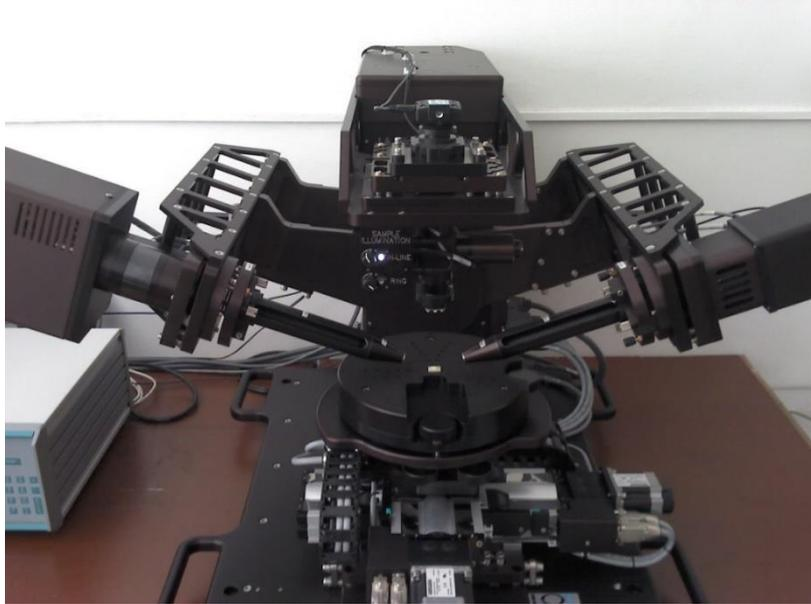
*Fig. 7 M-2000® Spectroscopic Ellipsometer (J.L. Woollam Co. Inc., USA)*
