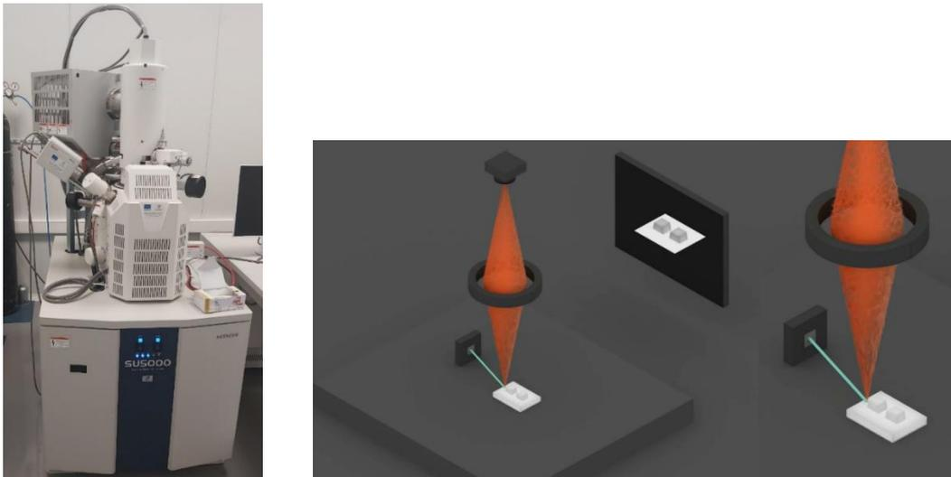
*Fig. 13 Scanning electron microscope SU5000 (HITACHI, Germany) and the principle of operation of SEM (Wikimedia Commons)*
