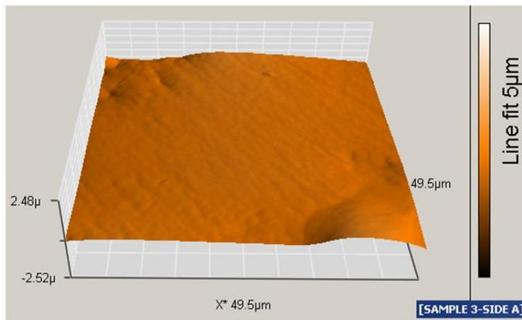
*Fig. 42 Test sample 10: Lithium disilicate press ceramics – glazed, treated with red diamond bur, polished with rubbers and diamond paste.*
