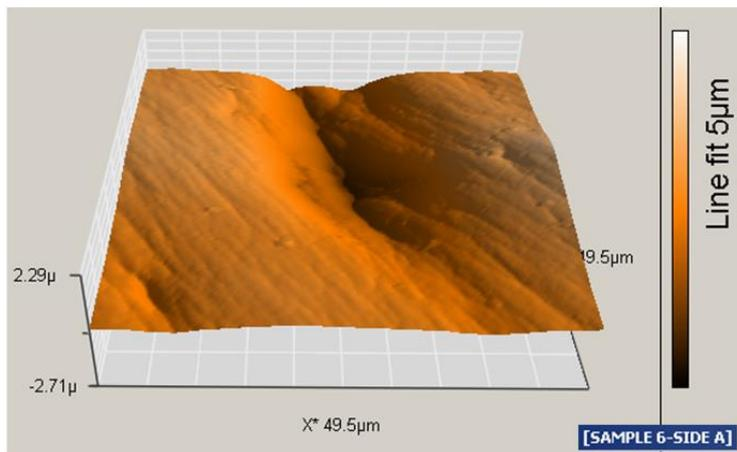
*Fig. 43 Test sample 11: Lithium silicate press ceramics – glazed, treated with green diamond bur, polished with rubbers and diamond paste.*
