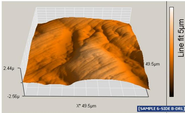
*Fig. 39 Test sample 7: Lithium silicate press ceramics – glazed, treated with green diamond bur, polished with rubbers.*
