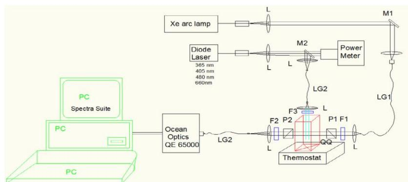
*Fig. 5 Optical scheme of an experimental setup for measuring optical parameters of ceramic materials using a microspectrophotometer and Spectra Suite software*
