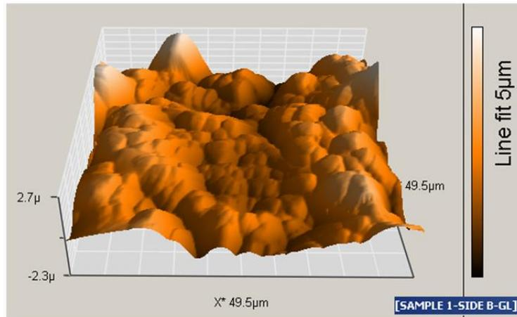
Fig. 34 Test sample 2: Lithium disilicate press ceramics (E.max Press) – laboratory polished
