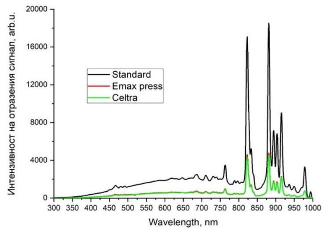
*Fig. 21 Reflection spectra of the studied ceramics in the range 200-1000 nm under illumination with a xenon lamp.*
