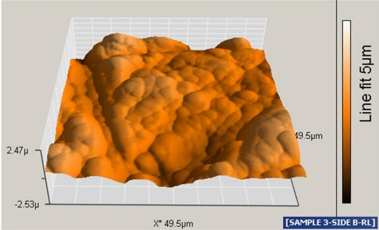
*Fig. 38 Test sample 6: Lithium disilicate press ceramics – glazed, treated with green diamond bur, polished with rubbers.*
