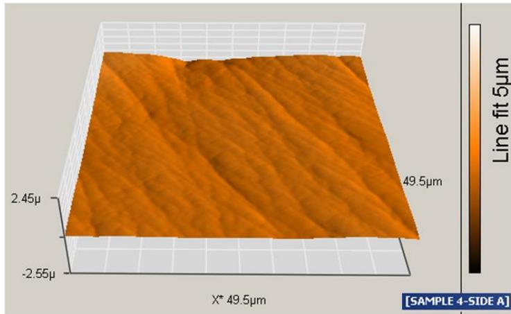
*Fig. 41 Test sample 9: Lithium silicate press ceramics – glazed, treated with red diamond bur, polished with rubbers and diamond paste.*
