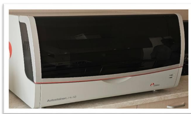
Figure 5. Dako Autostainer Link 48 used for immunohistochemical analysis at the Morphological Research Center, Medical University of Plovdiv.
